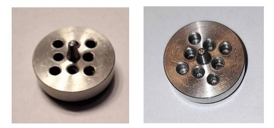
This makes a nice CNC project as demonstrated by Jordan Slavish's work and as seen on Patrick's web site! However, my approach is much simpler and involves only basic lathe and drill press work to make serviceable injector plates. Optionally, a milling machine with a rotary table attachment will do a beautiful job of precisely locating and drilling the orifice jet holes. A minor inconvenience of this approach is that the plate must be switched out to change jet configurations.
