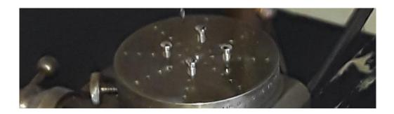
and I turned a special cylindrical fitting from 3/16" diameter aluminum to locate the injector part under the spindle by centering it on the depressor pin (photo below).
