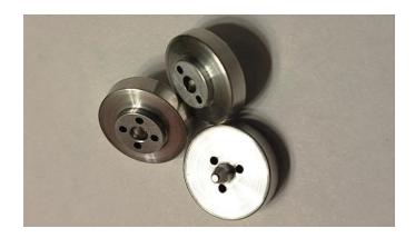
This is a set of procedures using a conventional "hand dialed" lathe, drill press and optional "hand dialed" milling machine to make simple "fixed-jet" injector plates for use with Patrick Carroll's revival of the *AeroTech* RMS 54/1280 Hybrid rocket motor. For more information see
